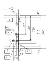
**Electric** Supply voltage: 400 V/3N ph/50/60 Hz Total Watts: 1.5 kW Water: Inlet water line size: 3/4" Incoming Cold/hot Water line 3/4"
